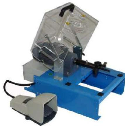
**Extérieur :** ESK 6, 8, 10, 13, 16, 19, 25, 32, 38, 50. **Intérieur :** ISK 13, 16, 19, 25, 32, 38, 50. Vitesse de rotation de 370 rpm.
